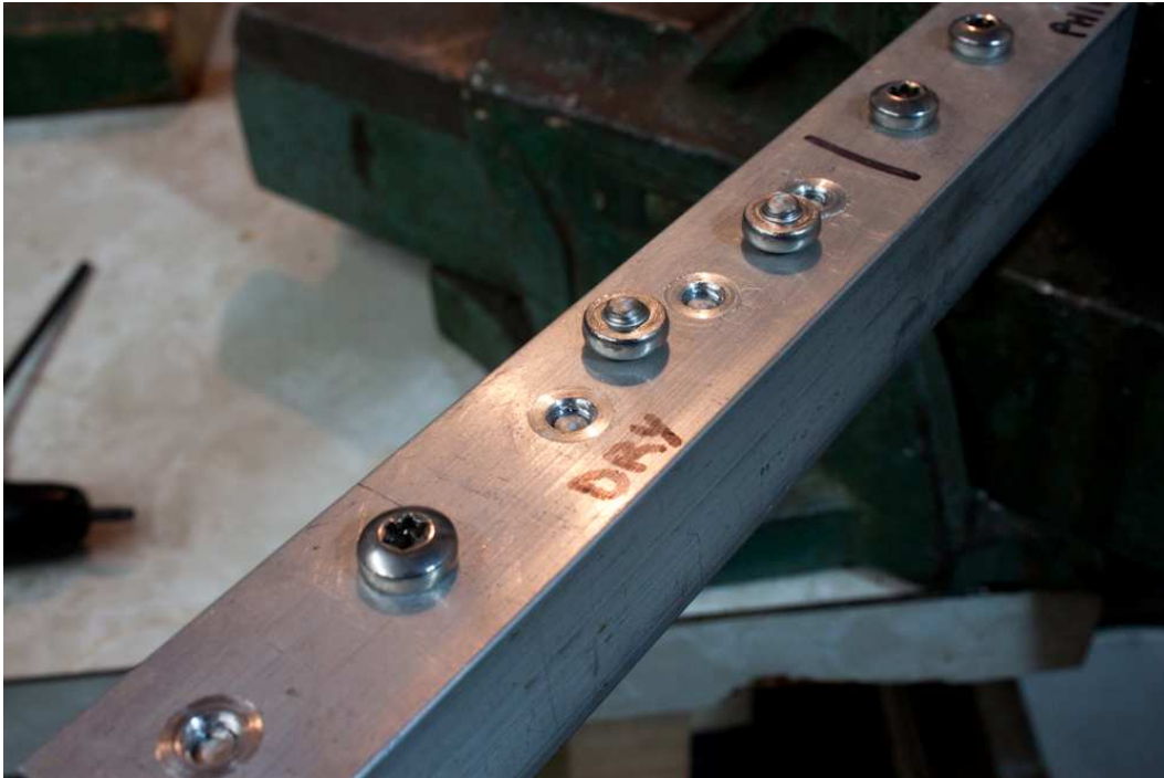
Bolt heads after dry full engagement test.
